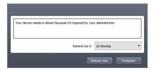
Users can restart the endpoint immediately by clicking 'Reboot now', or postpone it by picking a time in the 'Remind me in' drop-down.
