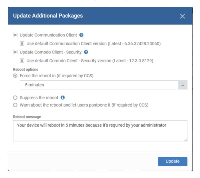
**Update Communication Client** - Only available for devices with an out-dated version of the communication client. As the name suggests, the communication client allows EM to send and receive updates to/from devices.
